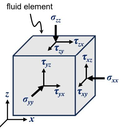
3. The **deviatoric** (viscous) stress arises when a fluid body is in motion. It can be approximated as a linear function of the strain rate tensor,  $e_{kl}$
