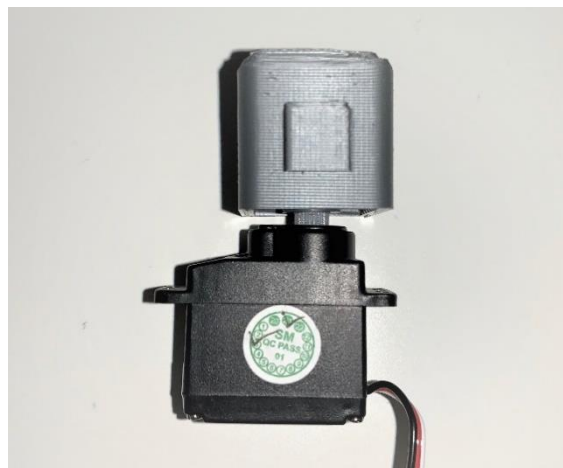
Figure 11: Servo motor and rotating cube (testing phase).
